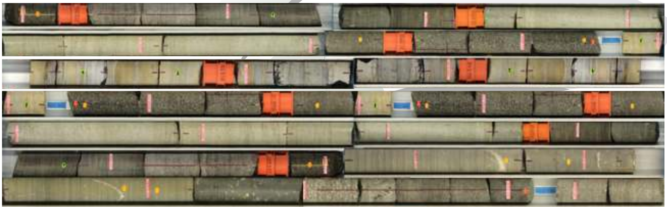
Compiled 2.0m tray projection displaying Core depth markers and Core Loss zones
