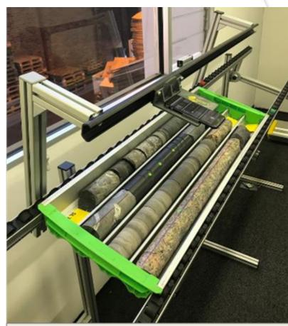
The tilting roller bed **WORK BENCH** with the attached camera accessory provides an ergonomic option allowing the operator to be seated when logging or photographing the core.
