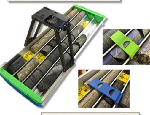
The **ALIGNMENT TOOLS** are used to rotate the core towards the camera, ensuring that the orientation line appears in the center of the channel.
